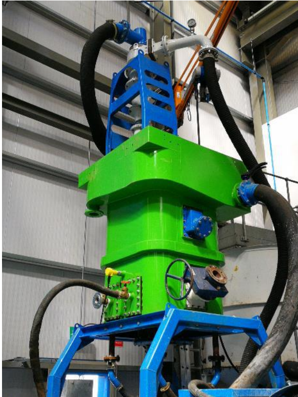
Laboratory built counter flow classification unit (CFCU) in CDE facility
