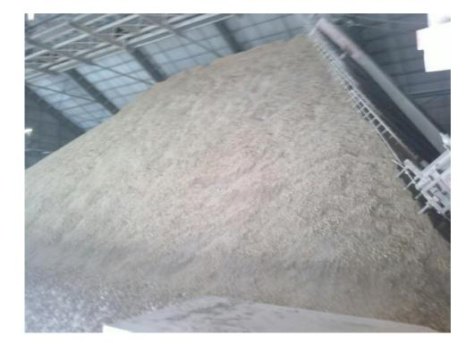
• Stacking of raw material including 15% demolition concrete sand and gravel
